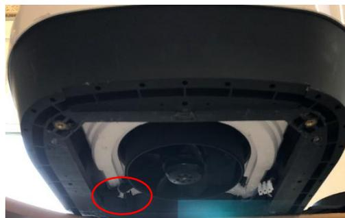
2.2 The sensor is zip tied together with the fresh air intake (the black tube)
