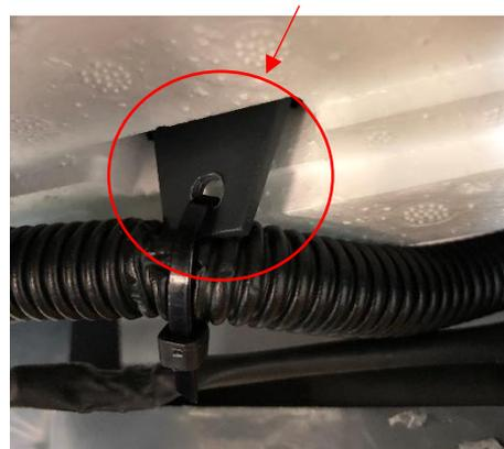
3.2 Put the inner mounting panel back again and screw in the bolts, you need to do that before you can place the RT sensor the right place:
